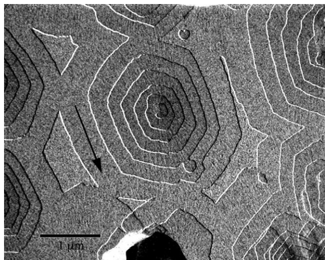
Fig. 1. Transmission electron micrograph of PCL 39 single crystals grown from toluene/ n -hexanol solution according to method M2. The arrows indicate the crystallographic b -axis of the different single crystals.
